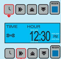
Time of day should only need to be set after power outages lasting more than 8 hours, if the battery has been depleted and a power outage occurs, or when daylight savings time begins or ends. If a power outage lasting more than 8 hours occurs, the time of day will flash on and off which indicates the time of day should be reset. If a power outage lasts less than 8 hours and the time of day flashes on and off, the time of day should be reset and the battery replaced. Type #2032 3V Lithium Battery
