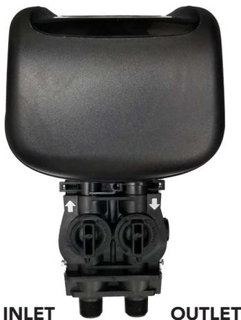
Your new system must be installed correctly. The inlet and outlet are shown in the picture. The arrows have been enhanced in the picture for easier identification. Significant damage to the system and your plumbing can occur if the system is installed backwards.
